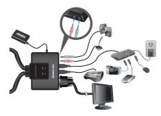
Connect a set of your molded KVM cable to each of your computers – DVI cable to the DVI output, USB cables to open USB ports from your computer, audio cable to your audio output and mic. cable to the mic. input.
